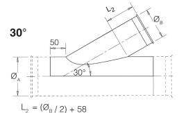
$\emptyset_{\scriptscriptstyle D}$  must be smaller than or equal to  $\emptyset_{\scriptscriptstyle A}$
