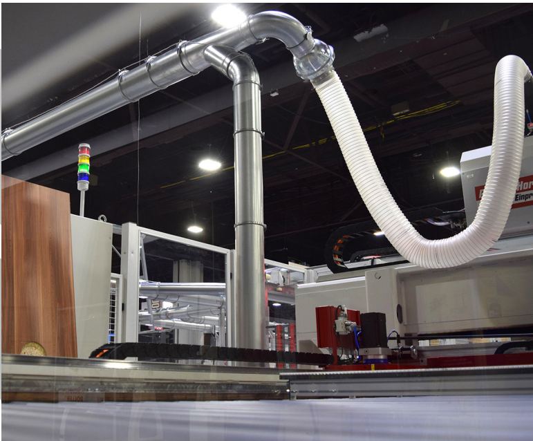
Above: A QF Ball Joint is shown in a QF duct line installed on woodworking machinery. Nordfab provides a full range of PU Hoses.
