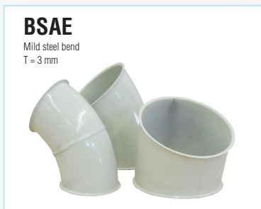
Order example: Bend Seg MS 3mm 800FB 90Deg R=1.5 RAL 7032
