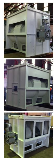
Important note: Fires and dust explosions can be caused by various ignition sources including sparks and optimum dust concentrations etc. We recommend fitting dust collectors with explosion vents and locating them outside of buildings to reduce the risk of damage to property and personnel in the event of an explosion or fire.
