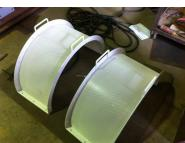
The rubber tips are easily replaceable from several locations around the rotary separator. The perforated screens can also be easily changed for different particle sizes. The gearbox is also easily changed as the shaft is supported by bearings at both ends of the machine.
