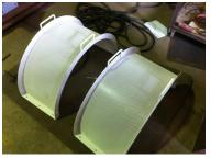
The rubber tips are easily replaceable from several locations around the rotary separator. The perforated screens can also be easily changed for different particle sizes. The gearbox is also easily changed as the shaft is supported by bearings at both ends of the machine.
