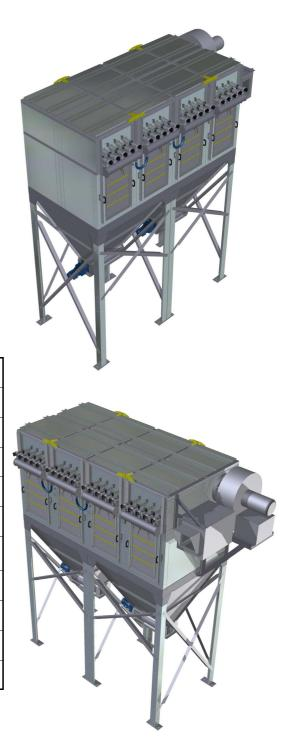
Important note: Fires and dust explosions can be caused by various ignition sources including sparks and optimum dust concentrations etc. We recommend fitting dust collectors with explosion vents and locating them outside of buildings to reduce the risk of damage to property and personnel in the event of an explosion or fire.
